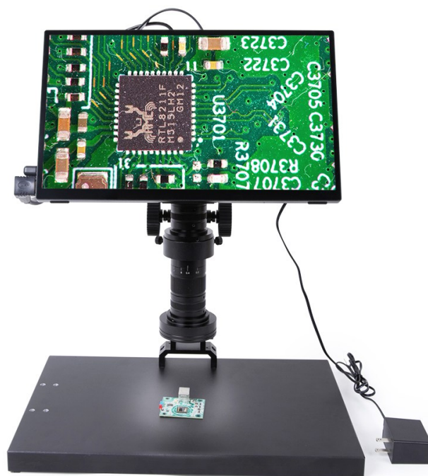
Figure 3-77 TPS-210A50(Stand)+TZM0480 (0.4x-8.0x Monocular Zoom Objective) +TXCAMLITE4K Camera(HDMI/USB Output CMOS Camera with Touch Function)+Touch Screen, the Touch Screen Is Fixed on the Fixing Block at the Front of the Camera through the Mounting Hole on the Built-in Bracket (Front View, Short HDMI Cable and USB Type A to Type C Data Cable Can Be Used to Connect the Camera and Touch Screen)
