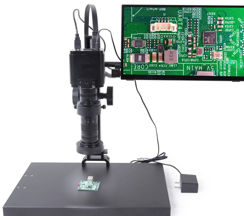
Figure 3-78 TPS-210A50-G(Stand)+TZM0480 (0.4x-8.0x Monocular Zoom Objective) +TXCAMLITE4K Camera(HDMI/USB Output CMOS Camera with Touch Function)+Touch Screen, the Touch Screen Is Fixed on the Cross Bar of Stand through the Mounting Hole on the Built-in Bracket (Front View, Short HDMI Cable and USB Type A to Type C Data Cable Can Be Used to Connect the Camera and Touch Screen)
