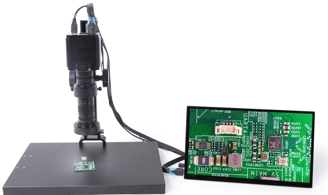
Figure 3-76 TPS-210A50(Stand) + TZM0480(0.4X~8X Monocular Zoom Objective) + TXCAMLITE4K(HDMI/USB Output CMOS Camera with Touch Function) + Touch Screen, the Touch Screen Can Be Tilted on the Table Through Its Own Stand (Long HDMI Cable and USB Type A To Type C Data Cable Are Required To Connect the Camera and Touch Screen)
