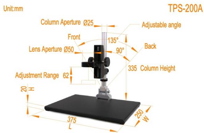
Figure 7-14 TPS-200A. TPS-200B can be obtained by rotating base B20A 90 degrees(B20B) and assembling it with bracket A20
