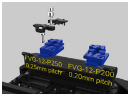
Easily exchangeable fiber guide V-grooves.
