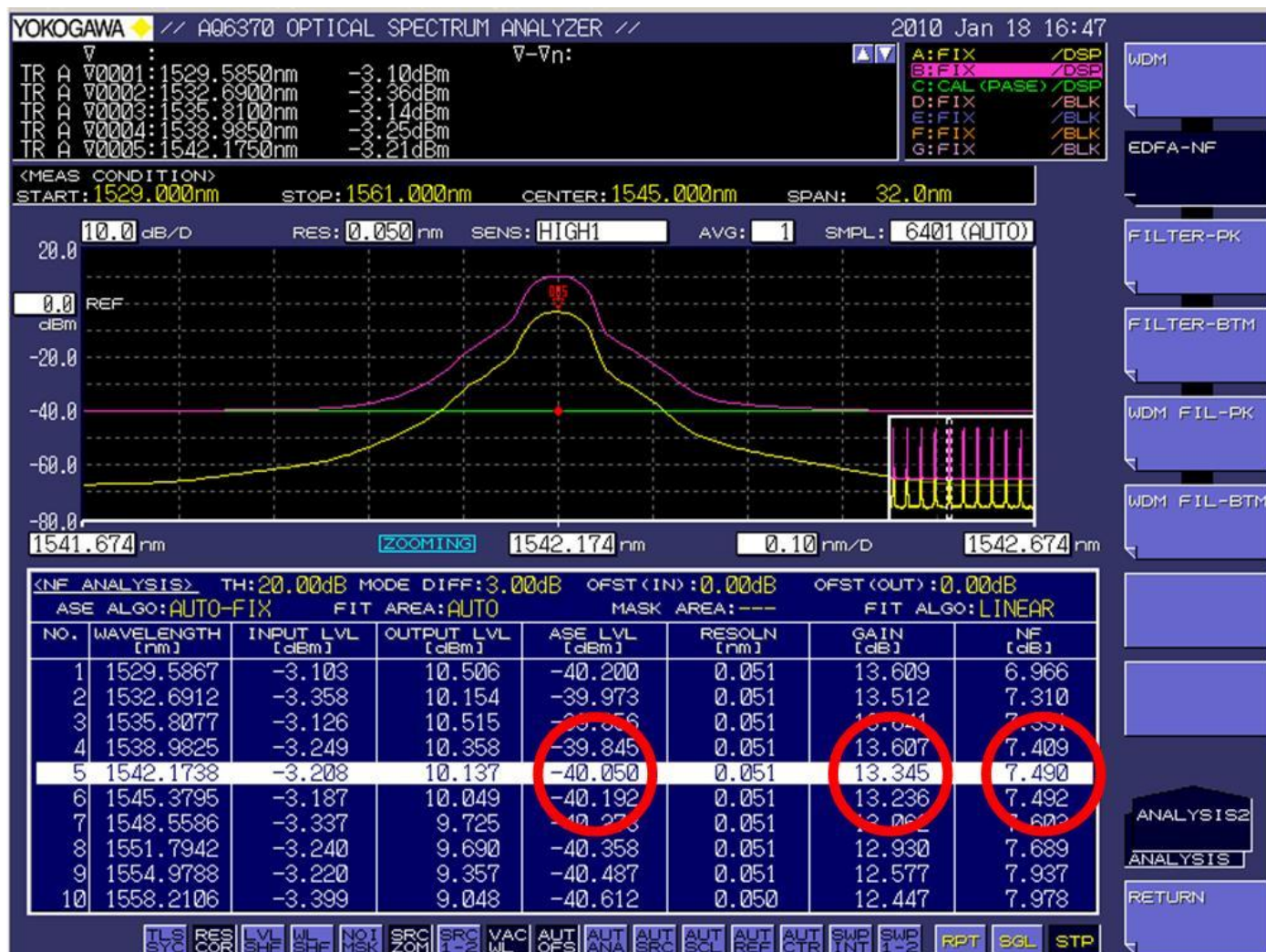
Figure 10 – The automated routine for optical amplifier analysis provides a table with the relevant parameters. Notice that the results of peak number 5 is in agreement with the manually obtained values.
