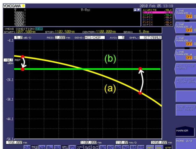
Figure 5. - Recorded OSA trace (a) is converted to the power density spectrum (b) by dividing the measured power by the local effective resolution
