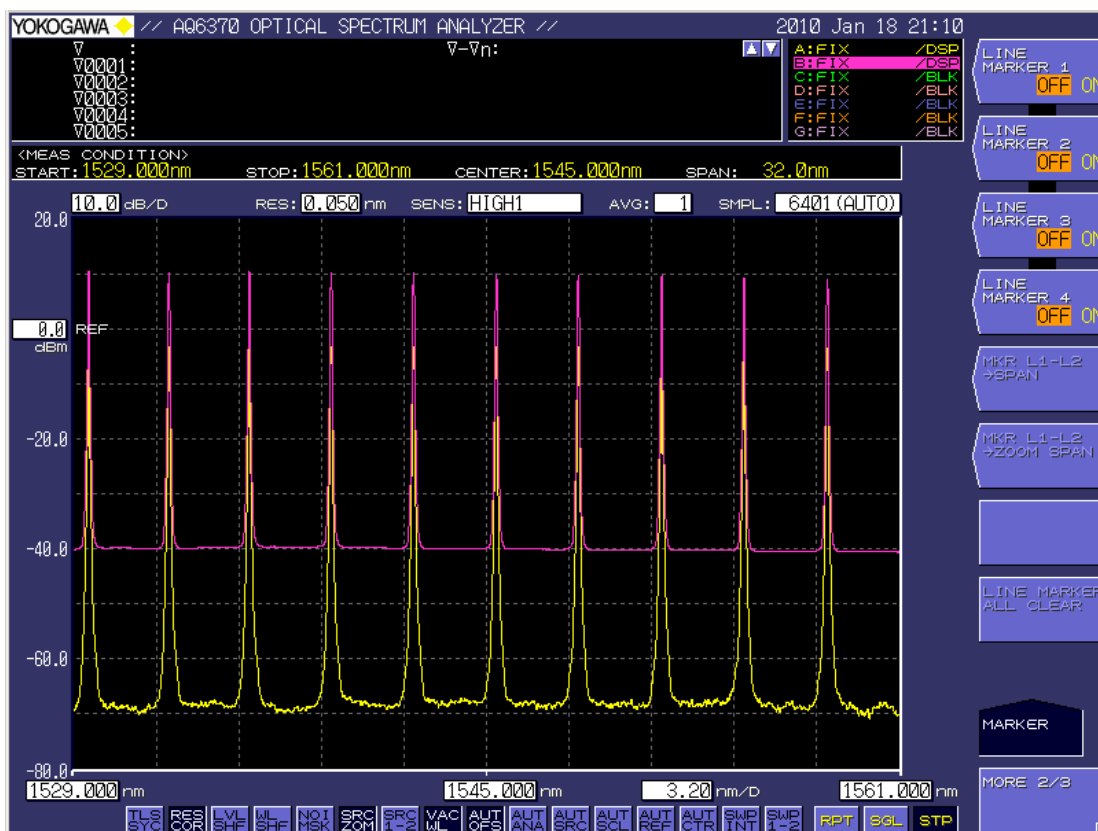
Figure 4 – Typical obtained measurement result showing two traces; one before amplification (yellow) and one after amplification (purple).
