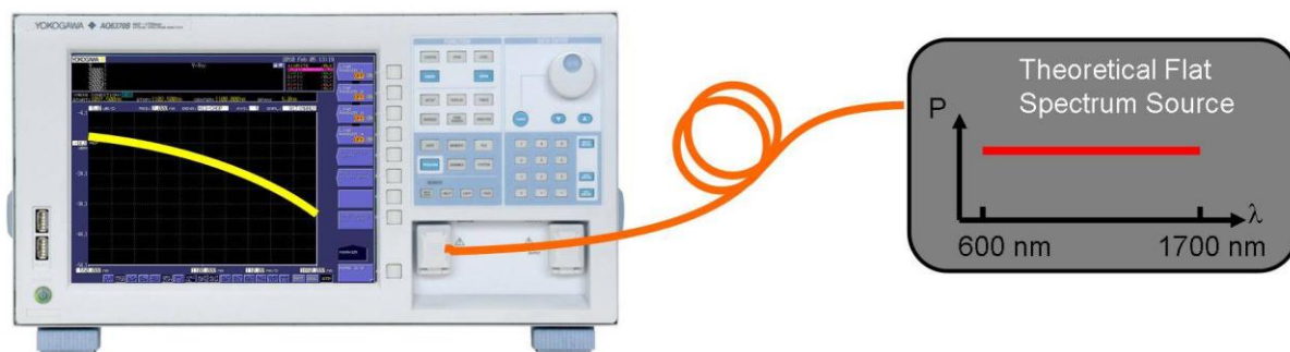
Figure 4. - Absolute power display: the recorded spectrum of a perfectly flat spectrum is dropping towards longer wavelengths
