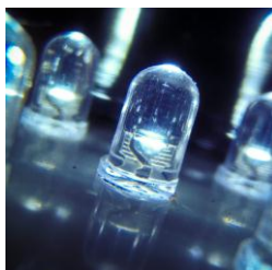
LEDs in pulsed operation to achieve a higher brightness
