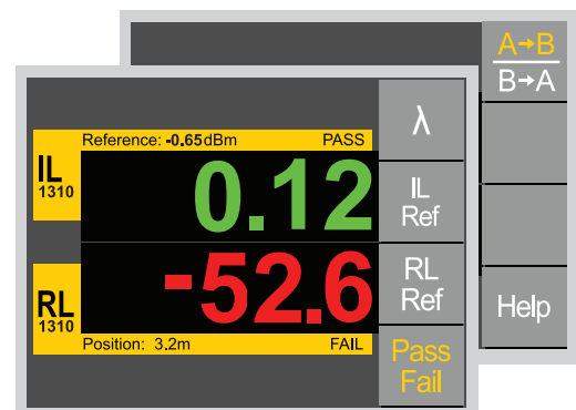
Figure 3: OP940 ILRL Measurement Mode with direction switching functionality (A-B/B-A)
